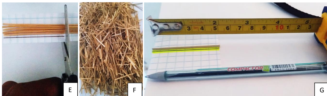
Figure 1: Extraction and cutting of fibers, (A) Bambuzal, (B) (C) and (D) Extraction and manual production, (E) Cutting of fibers on graded paper, (F) Cut polymeric fibers, (G) Fiber Length.
