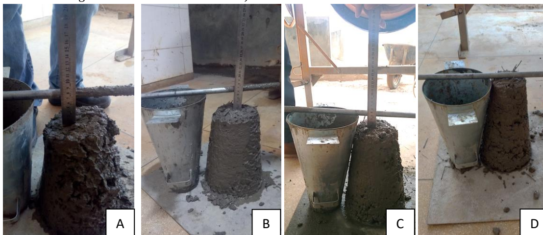
Figure 3: Cone Trunk Discharge Test, (A) Conventional Concrete, (B) Concrete with 3% Bamboo Fiber Addition, (C) Concrete with 4% Bamboo Fiber Addition, (D) Concrete with 5% added bamboo fibers.
