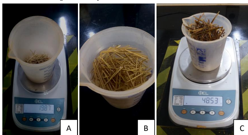
Figure 2: Determination of water content absorbed by bamboo fibers, (A) Weight in dry natural state, (B) Immersion in water, (C) Weight of fibers (post) immersion.
