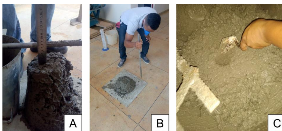
Figure 2: mixture characterization procedures, (A) Slump test performed on the trace, (B) workability verification test, (C) consistency test.
